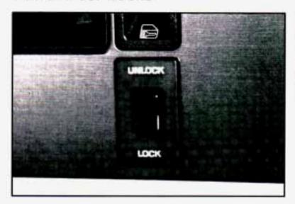
If your vehicle has power door locks, push the power door lock switch to lock or unlock all the doors at once.
